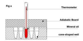
The display shows usually 1 - 2 K less in comparison to what is measured with the thermometer in the hole. This is consciously done because the SCBIs being put in are not totally covered from the aluminum block and the temperature inside the SCBI is also typically 1 - 2 K below the aluminum block temperature.
