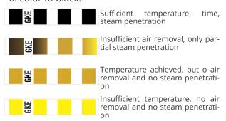
Colour change of a standard indicator strip. If using an indicator strip for prion programs the initial colour is pink.
