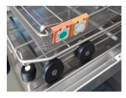
The picture on the left shows two indicators after having passed a cleaning cycle. The indicator on the right hand side had been stored under correct conditions and is washed off completely. The indicator on the left-hand side had been taken from the cabinet shown above. The indicator colour is fixed due to the chemical reaction of the disinfectant vapor with the indicator substance and cannot be washed off any more.
